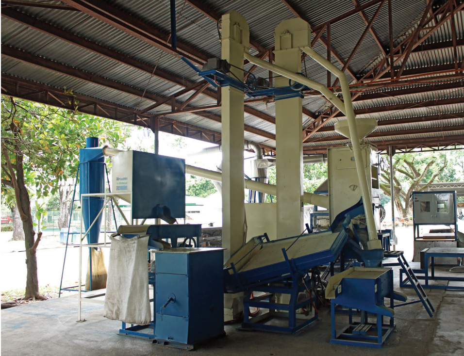
Retrofitted compact rice mill for production of both well-milled and brown rice
